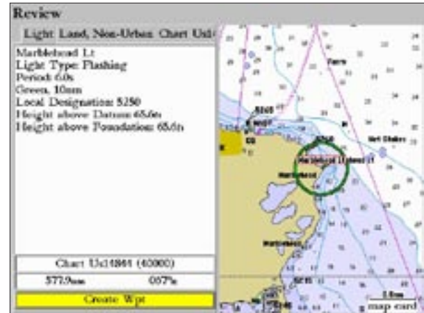
Using a map item to create a new waypoint. (BlueChart data shown.)
